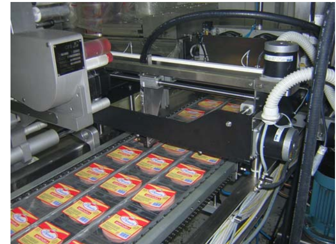
Print across multiple lanes of packaged food or other products to code multiple packages in one movement
