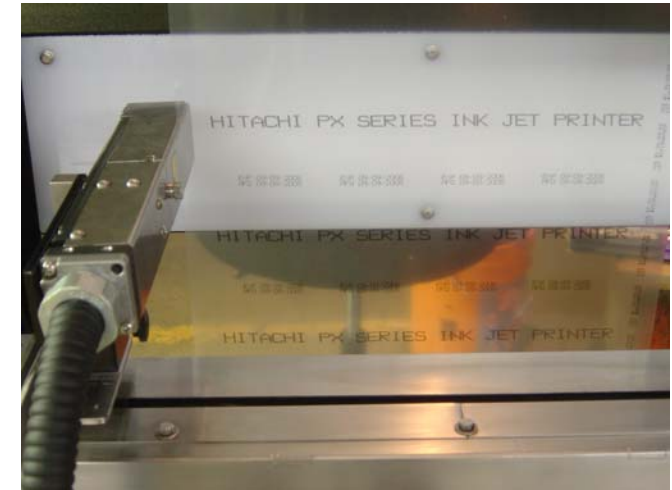
Print onto plastic film in both movement directions to increase speed or print alternating information
